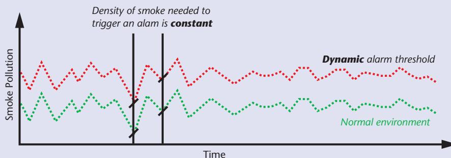
ClassiFire® dynamically adjusts the detector sensitivity to match changes in the normal environmental smoke density, thus the amount of smoke needed to generate an alarm remains constant, irrespective of environmental conditions.
